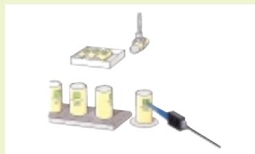
Used for aligning directions for packaging by detecting delicate color differences or very fine marks.
