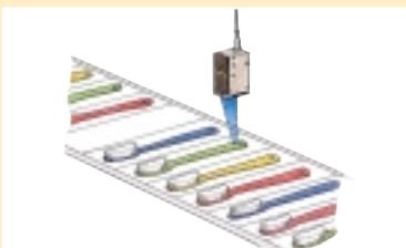
Sorts toothbrushes by the color of their handles. Stable detection can be obtained without being influenced by changes in brightness of sensing objects.
