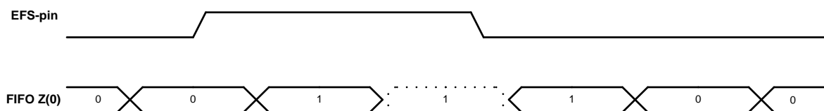
Figure 35: Timing diagram for external FIFO synchronization.
