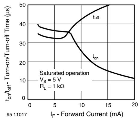
Fig. 16 - Turn-on/off Time vs. Forward Current
