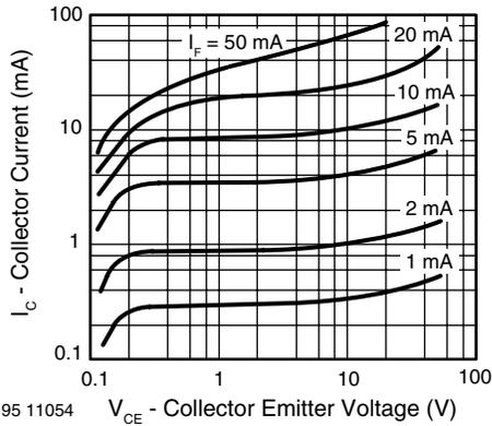
Fig. 12 - Collector Current vs. Collector Emitter Voltage
