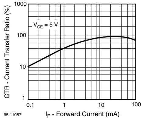
Fig. 15 - Current Transfer Ratio vs. Forward Current
