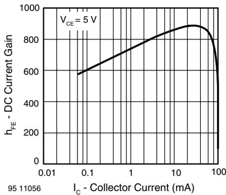
Fig. 14 - DC Current Gain vs. Collector Current
