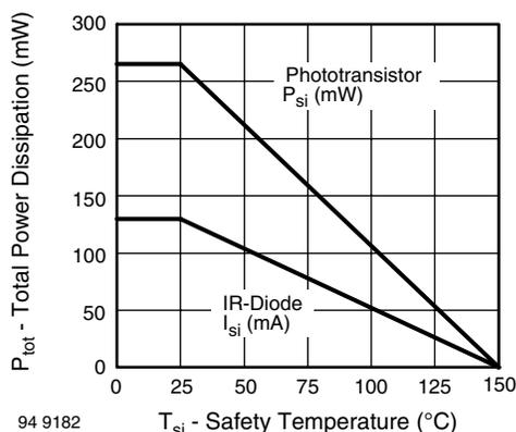
Fig. 1 - Derating Diagram
