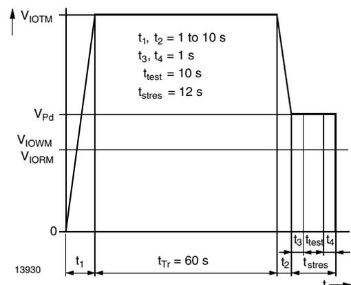
Fig. 2 - Test Pulse Diagram for Sample Test According to
