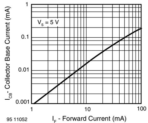
Fig. 10 - Collector Base Current vs. Forward Current
