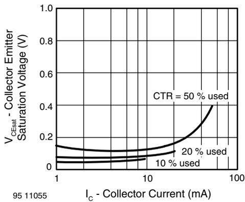
Fig. 13 - Collector Emitter Saturation Voltage vs. Collector Current
