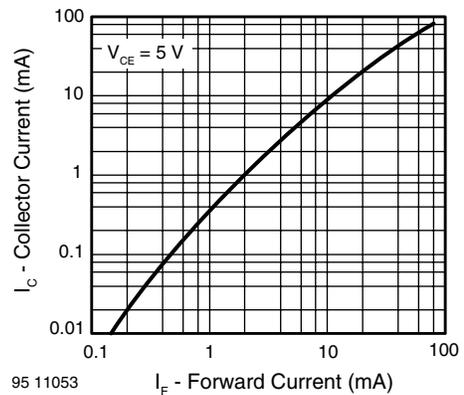
Fig. 11 - Collector Current vs. Forward Current
