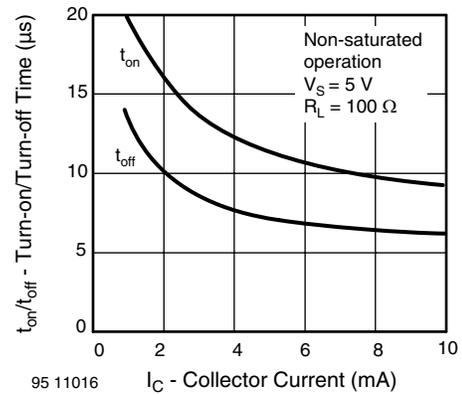
Fig. 17 - Turn-on/off Time vs. Collector Current
