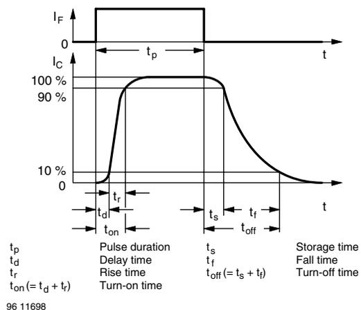
Fig. 5 - Switching Times
