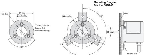
Material: SPCC Thickness: 3.2 Applicable model: E6B2-C
