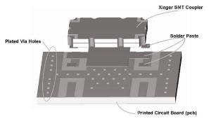
Figure 4: Mounting Features Example
