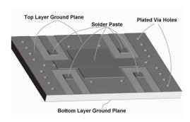
Figure 2: Solder Paste Application
