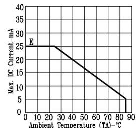
Fig5. MAX. ALLOWABLE DC CURRENT VS. AMBIENT TEMPERATURE.
