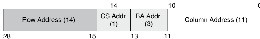
Figure 2-8. Mapped Address for the Example
