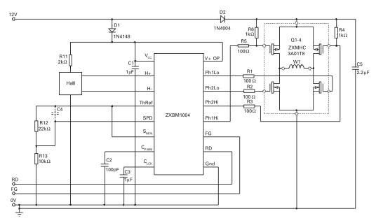
Figure 4: Typical circuit for constant speed operation
