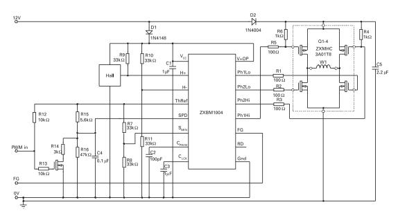
Figure 2: Typical circuit for external PWM controlled speed
