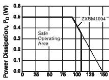
Ambient Temperature, T<sub>▲</sub> (°C) **Power Derating Curve**
