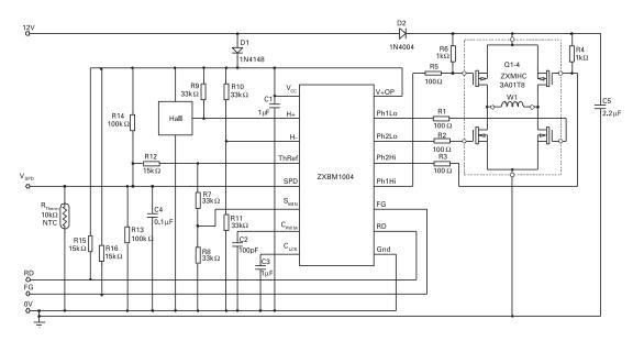
Figure 1: Typical circuit for thermistor controlled speed
