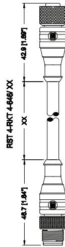
Actuator/sensor cordset, double-ended, M12, 3-4-poles, male straight to female 90° connector with self-locking thread and molded cable.
