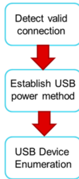
Figure 62. Flow of DFP to UFP Configuration
