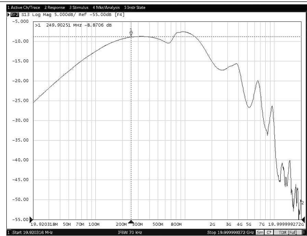
Figure 32. Off-State Data-Switch Isolation vs Frequency (TPS25830-Q1)
