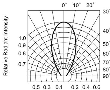
FIG.6 RADIATION DIAGRAM
