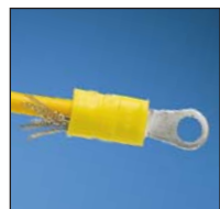
Bent Back Strands
