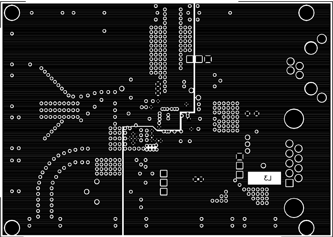
Figure 77. Evaluation Board Power—Layer 3
