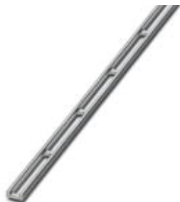
Cross connection rail, for fixed bridging of identical inputs and outputs, made of Cu, nickel-plated, 1 m long
