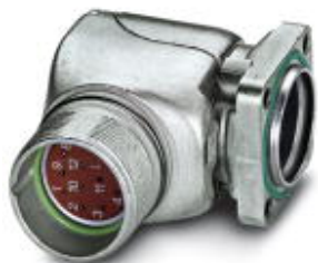
Device connector, front mounting, angled rotatable, Screw locking, M23, number of positions: 17, type of contact: Socket, Crimp connection, Axial O-ring, 4x Ø 3.2, shielded: yes, flange dimensions: 28 mm x 28 mm
