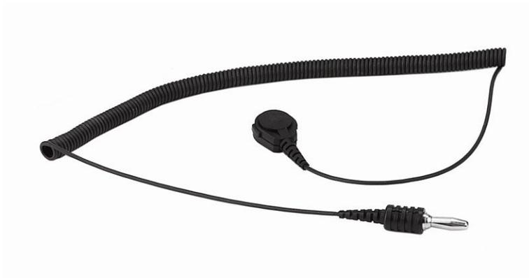
The 4600 Series Coil Cord is for use with Single-Wire Wrist Straps and SCS Workstation Monitors. Coil Cord features a segmented strain relief and a single bundle of tinsel conductors which provide long cord life and easy movement. Having a 1 megohm current limiting resistor (at the end to attach to the wristband), the Coil Cord meets the resistance requirements of ANSI/ESD S20.20, EIA 625. Alligator clip is included. Made in China.
