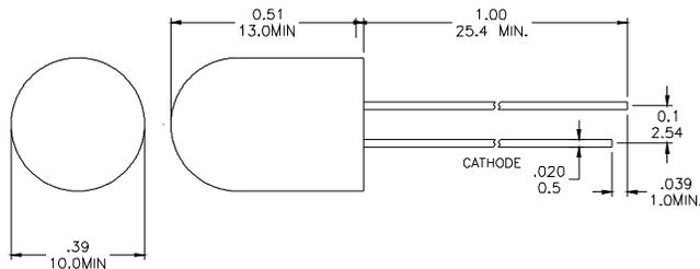
\* Tolerance :  $\pm \frac{0.01}{0.25}$       Unit :  $\pm \frac{\text{inch}}{\text{mm}}$
