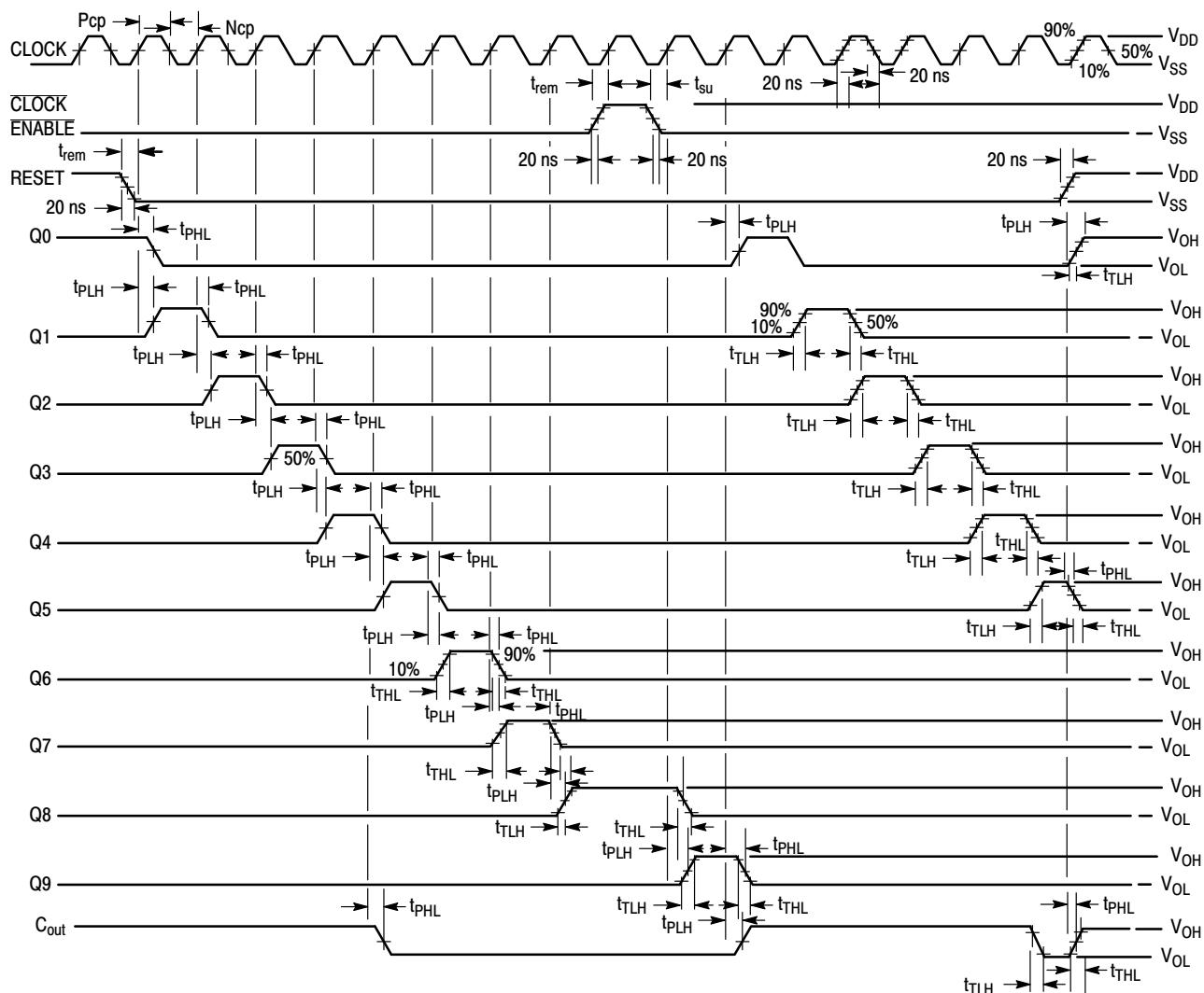
**Figure 4. AC Measurement Definition and Functional Waveforms**
