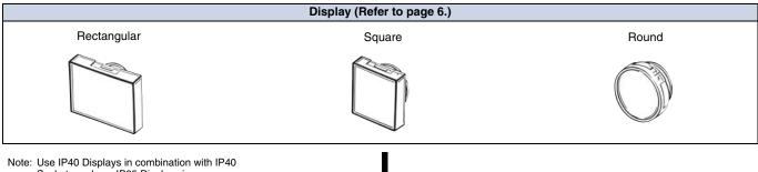
Note: Use IP40 Displays in combination with IP40 Sockets and use IP65 Displays in combination with IP65 Sockets. The Display has a legend plate built in.
