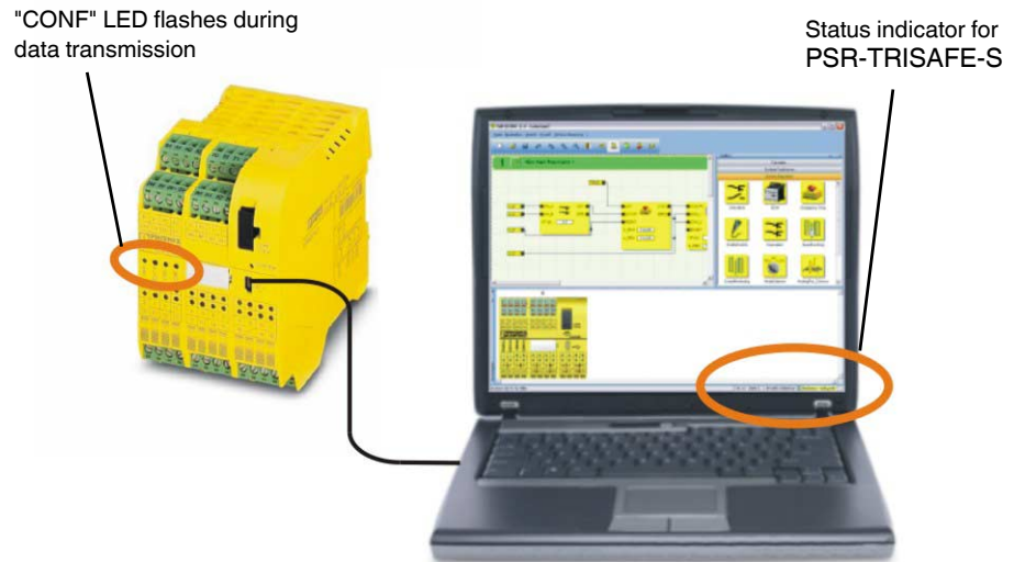
Figure 5-4 USB connection between PC and safety module
