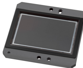
Figure 1. KAI-43140 CCD Image Sensor
