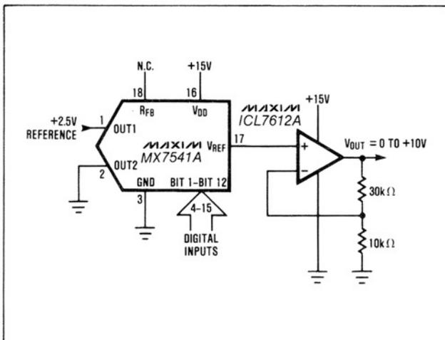
Figure 6. Single Supply Operation Using Voltage Mode
