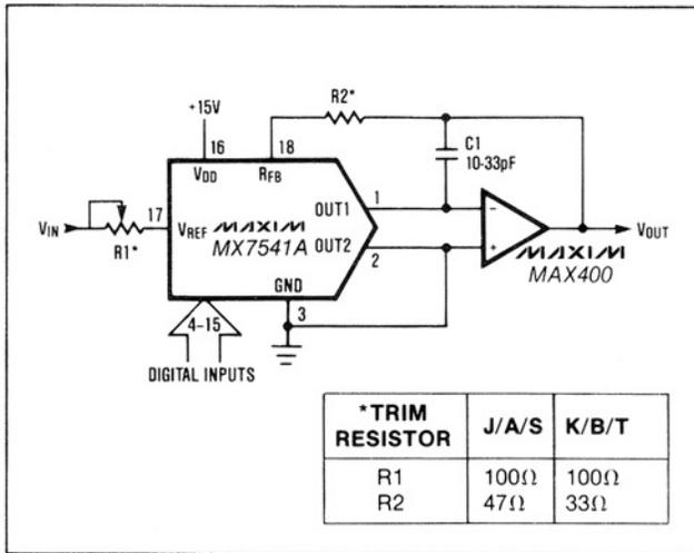
Figure 4. Unipolar Binary Operation
