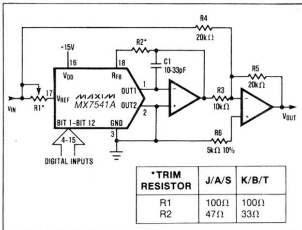
Figure 5. Bipolar Operation (4-Quadrant Multiplication)
