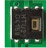
Relative humidity depends on temperature. To get the most accurate measurements from HTU21D click™, it's important to keep the sensor at the same temperature as the environment in which you want to measure the humidity.
