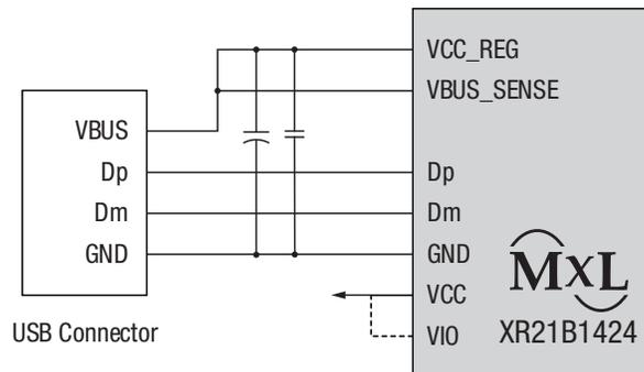
Figure 1: Bus-Powered Mode
