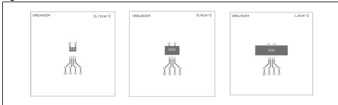
Figure 30. SO-8 PC board
