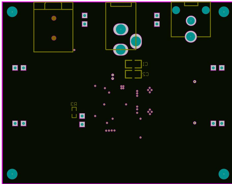
Figure 5. Board Component Placement Guide -Bottom Layer
