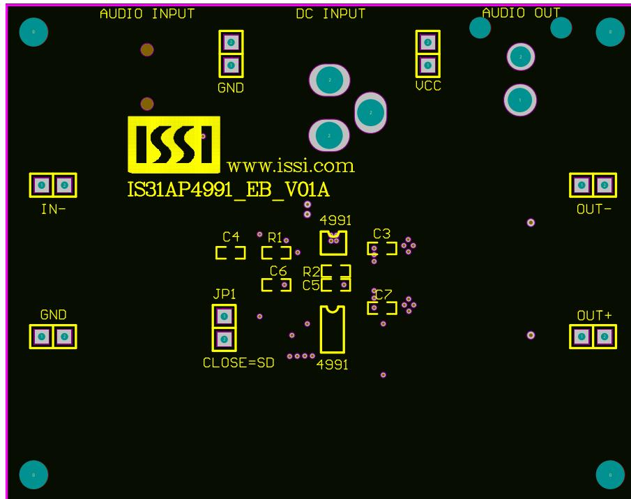
Figure 3. Board Component Placement Guide - Top Layer
