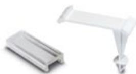
Phoenix module marker carrier, for labeling modules and PCBs, for hole diameter 3.9 to 4.1 mm, thickness of wall or board 1.5 - 2.0 mm, labeling with insert strips ESL, EST or ES/LP-BW-GB, lettering field: 29 x 8 mm
