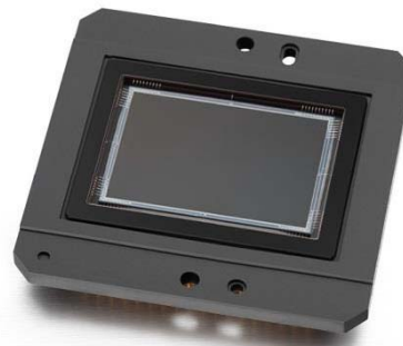
Figure 1. KAI-16050 CCD Image Sensor
