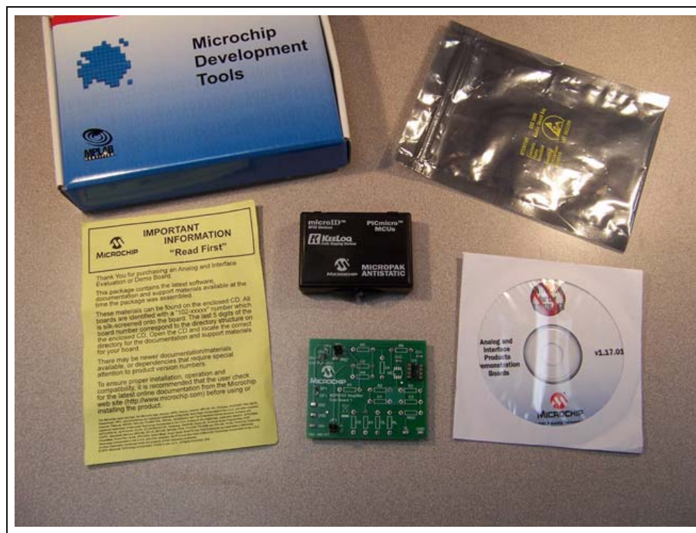
FIGURE 1-1: MCP6XXX Amplifier Evaluation Board 1 Kit.
