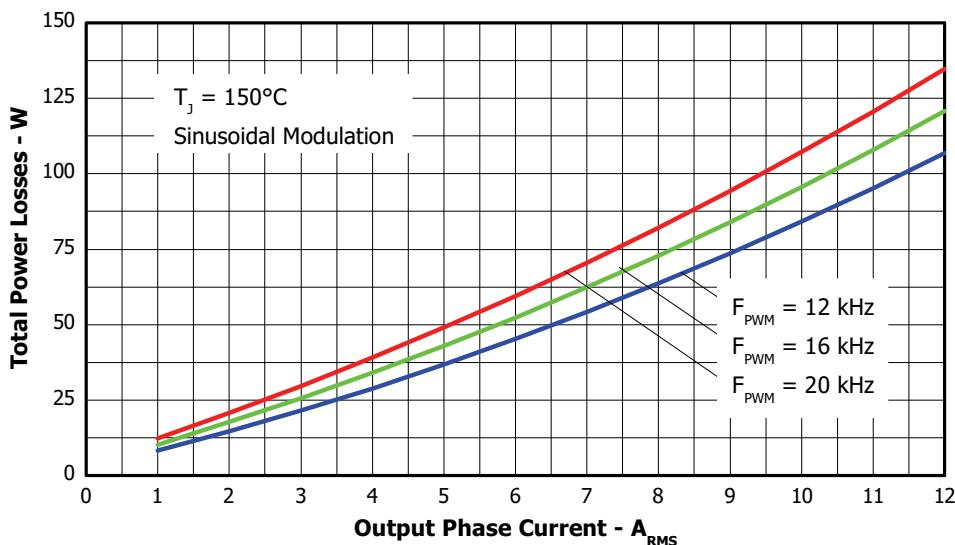
Figure 6. Total Power Losses vs. Output Phase Current, Sinusoidal modulation
