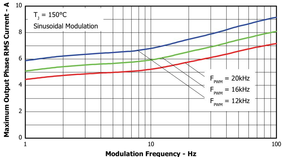
Figure 4. Maximum Sinusoidal Phase Current vs. Modulation Frequency
