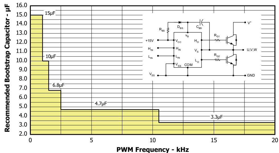
Figure 10. Recommended Bootstrap Capacitor Value vs. Switching Frequency
