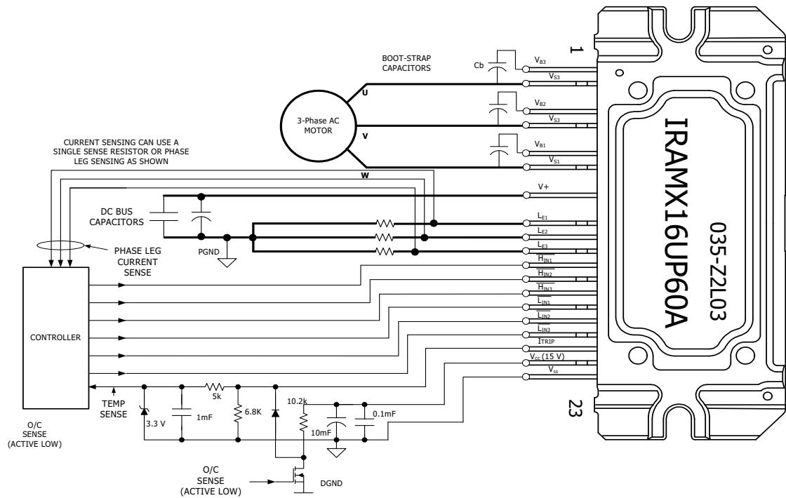
1. Electrolytic bus capacitors should be mounted as close to the module bus terminals as possible to reduce ringing and EMI problems. Additional high frequency ceramic capacitor mounted close to the module pins will further improve performance.
