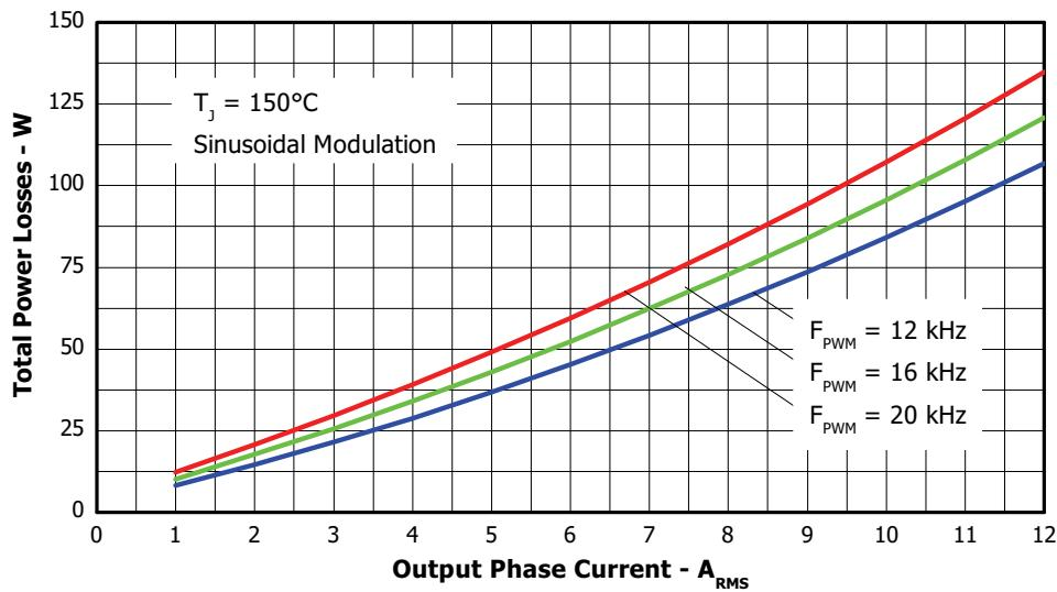
Figure 5. Total Power Losses vs. PWM Switching Frequency, Sinusoidal modulation
