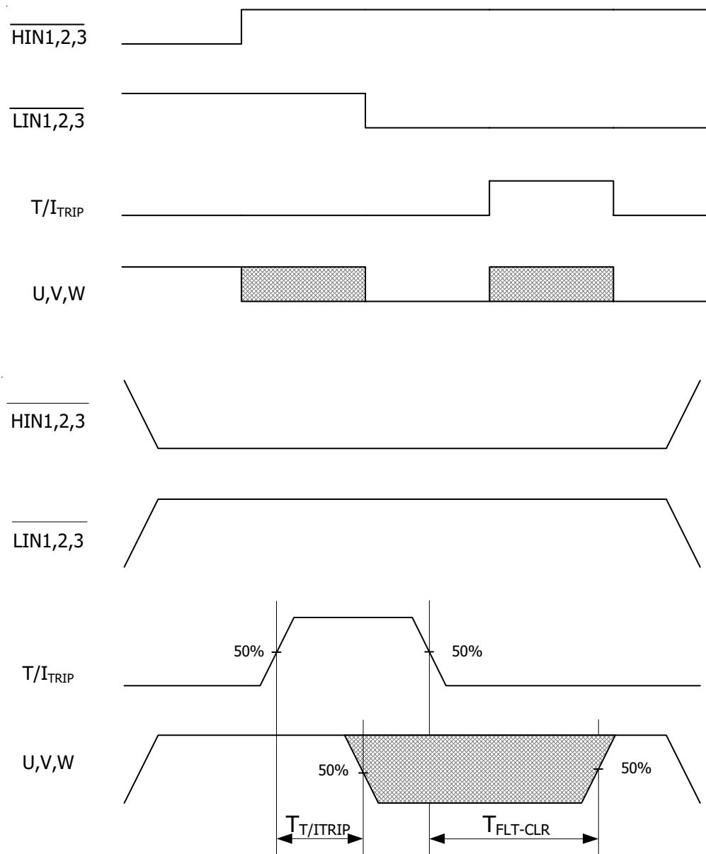
Note 5: The shaded area indicates that both high-side and low-side switches are off and therefore the half-bridge output voltage would be determined by the direction of current flow in the load.
