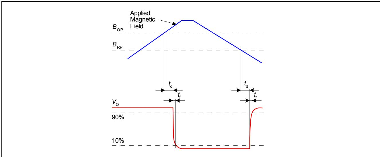
Figure 3 Timing diagram
