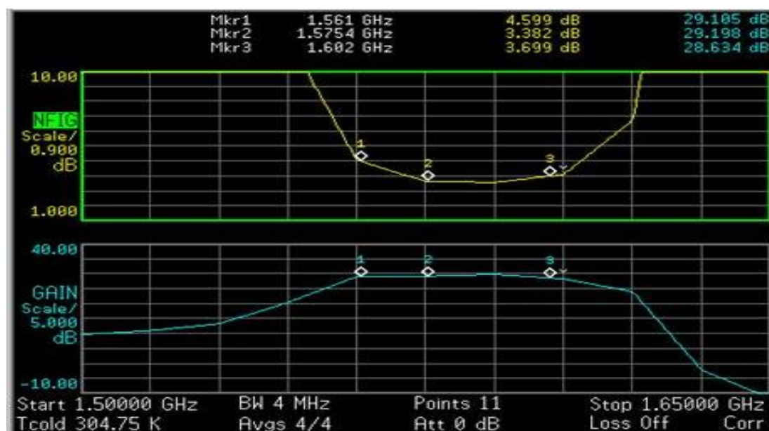
LNA Gain and Noise Figure @ 3.0V
