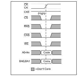
Figure 8 — Mode Register Set Command
