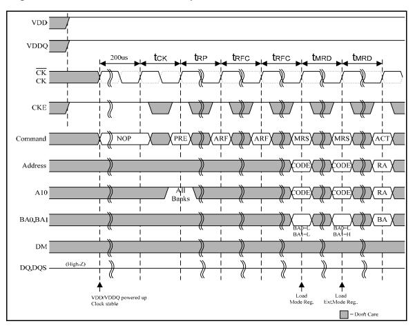
Figure 5 — Initialization Waveform Sequence
