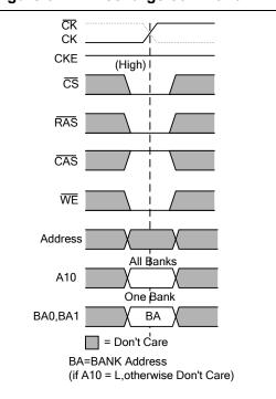
Input A10 determines whether one or all banks are to be precharged. In case where only one bank is to be precharged, inputs BA0,
