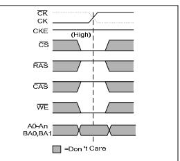
Figure 21 — Burst Terminate Command
