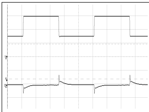
Figure 7: AGF800-48S28-6L Transient Response 25%~50%~25% load change, 0.1A/uS slew rate, Ch 1: Io (5A/div) Ch 2: Vo (500mV/div)
