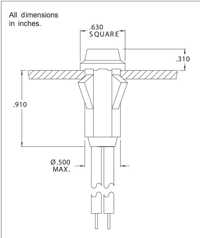
Mounting: Will snap-fit into Ø.500/.505 hole in panels .020/.100 thick. Push-on speednut SN0461 also available. Mounting hole pattern on page SP2.
