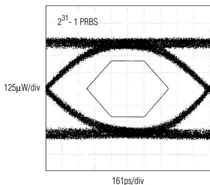
EYE DIAGRAM (622Mbps, 1300nm LASER, 470MHz FILTER)
