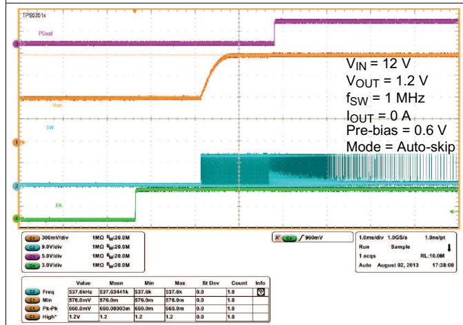
Figure 27. Auto-Skip Mode Shutdown Operation
