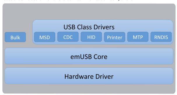
The different available hardware drivers, the USB class drivers, and the bulk communication component are additional packages, which can be combined and ordered as they fit to the requirements of your project. Normally, emUSB consists of a driver that fits to the used hardware, the emUSB core and at least one of the USB class drivers.
