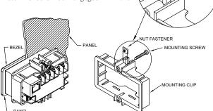
farthest forward slot possible. To achieve a proper seal, tighten the latch screws evenly until the unit is snug in the panel (Torque to approx. 28 to 36 in-oz [0.202 to 0.26 N-m]). Do not over-tighten the screws.
