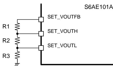
The VOUT maximum voltage ( $V_{VOUTH}$ ) and VOUT minimum voltage ( $V_{VOUTL}$ ) can be calculated using the formulas below.
