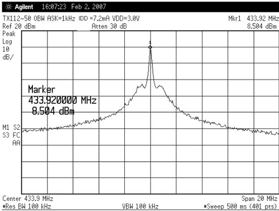
**RF Spectrum 2<sup>nd</sup> Harmonic; Fundamental at 433.92 MHz**
