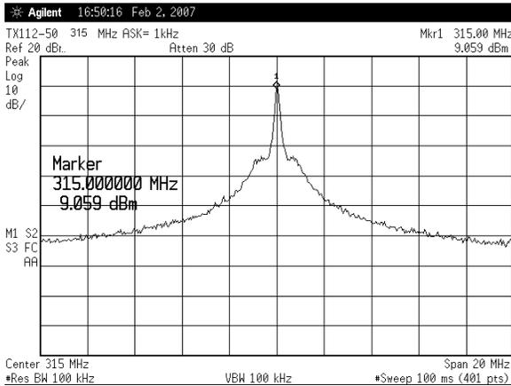
**RF Spectrum 2<sup>nd</sup> Harmonic; Fundamental at 315 MHz**
