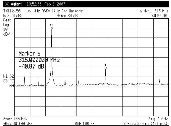
**RF Spectrum 3<sup>rd</sup> Harmonic; Fundamental at 315 MHz**
