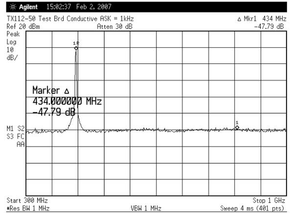
**RF Spectrum 3<sup>rd</sup> Harmonic; Fundamental at 433.92 MHz**
