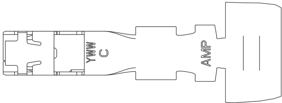
△ MATERIAL: 0.30 THICK COPPER ALLOY, PREPLATED WITH 0.0008 MINIMUM THICK REFLOW TIN OR BRIGHT TIN (ELV COMPLIANT).
