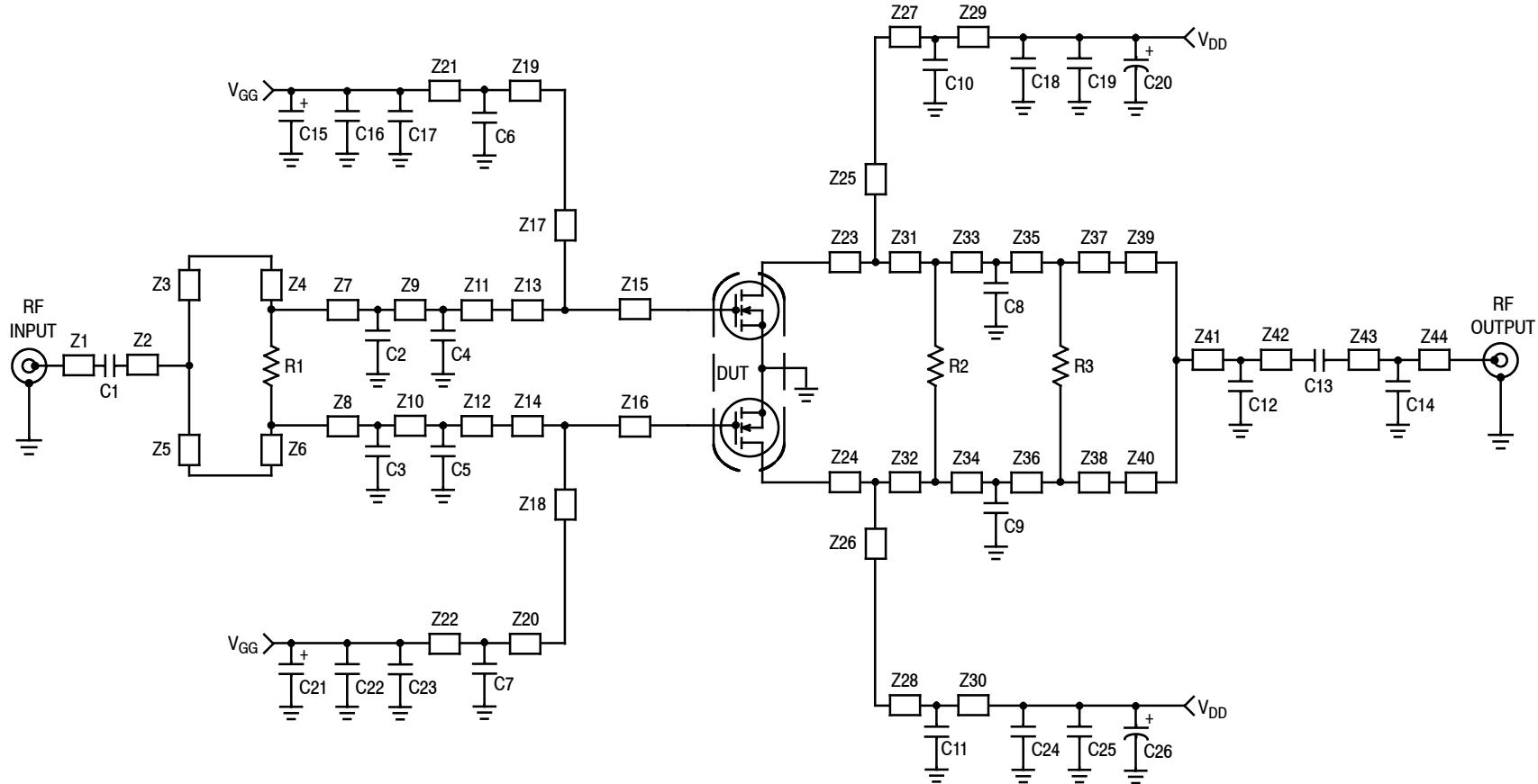
Figure 11. MRF8VP13350N Narrowband Test Circuit Schematic — 1300 MHz
