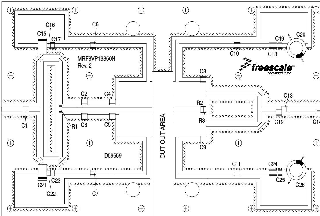
Figure 10. MRF8VP13350N Narrowband Test Circuit Component Layout — 1300 MHz
