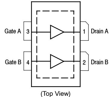
**Figure 1. Pin Connections**
