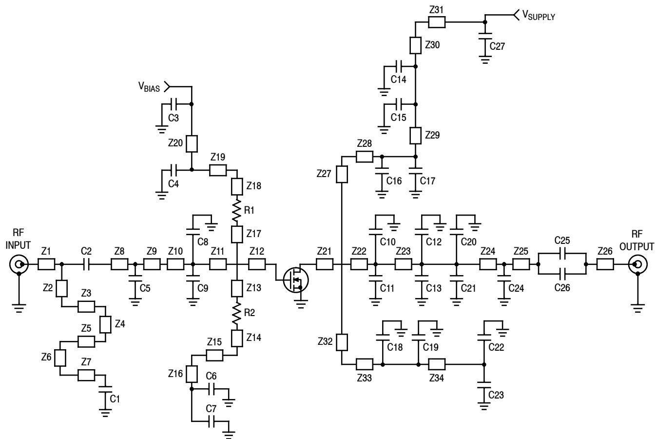
**Figure 5. MRF8VP13350N Reference Circuit Schematic — 915 MHz**
