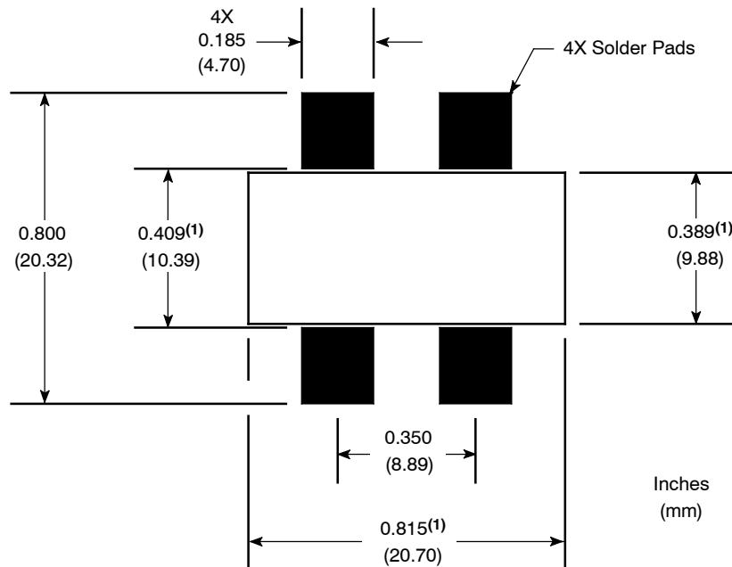
1. Slot dimensions are minimum dimensions and exclude milling tolerances.
