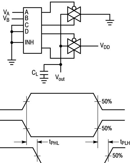
**Figure 9. Propagation Delay, Any Pair of Address Inputs to Output**
