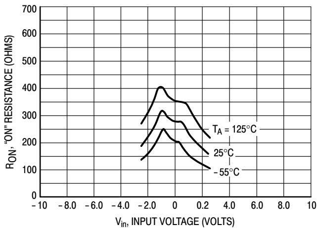
**Figure 12.**  $V_{DD} = 2.5$  V,  $V_{SS} = -2.5$  V
