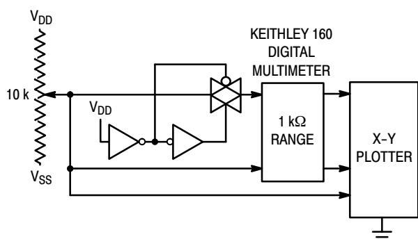
**Figure 8. Channel Resistance ( $R_{ON}$ ) Test Circuit**
