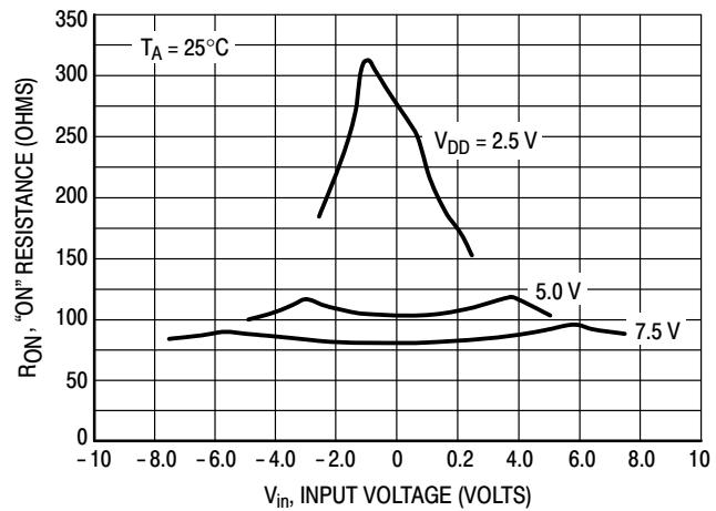
**Figure 13.** Comparison at  $25^\circ\text{C}$ ,  $V_{DD} = -V_{SS}$
