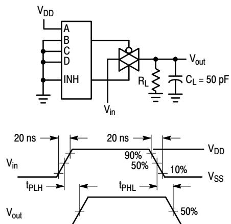
Figure 3. Propagation Delay Test Circuit and Waveforms  $V_{in}$  to  $V_{out}$
