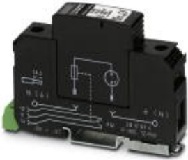
Surge arrester type 2, consisting of base element with remote indicator contact and protective plug with N-PE total current spark gap for mounting on NS 35/7.5, housing width: 17.5 mm (1 Div.)
