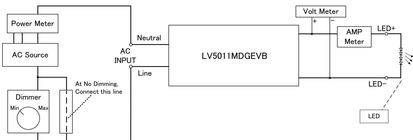
**Figure1.** LV5011MDGEVB Recommended Test Set Up
