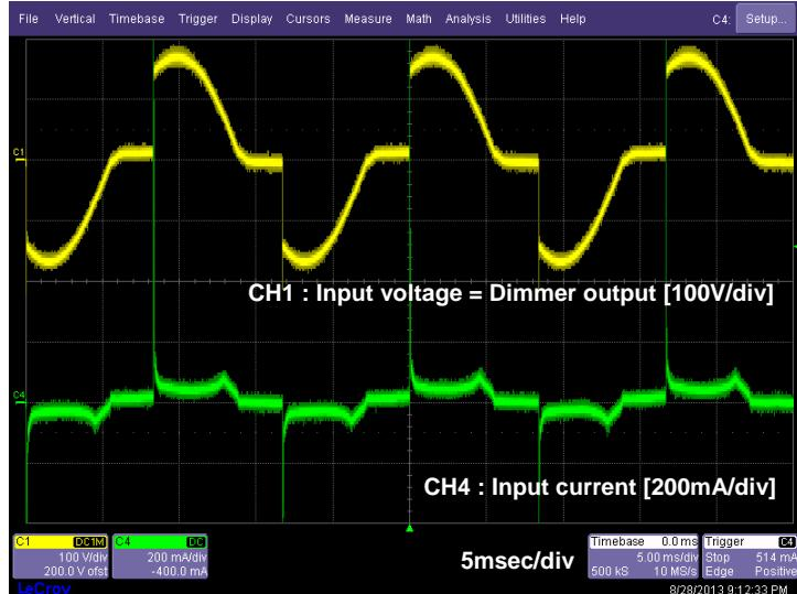
**Figure10.** Dimming operation waveform at
