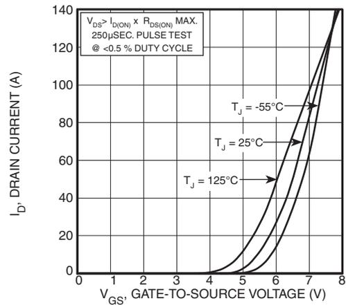
Figure 4, Transfer Characteristics
