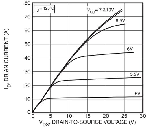
Figure 2, Output Characteristics
