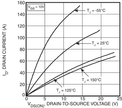
Figure 1, Output Characteristics
