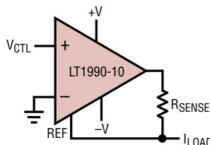
$I_{LOAD} = 10 \cdot V_{CTL}/R_{SENSE} \leq 3mA$
