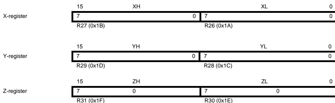
Figure 6-5. The X-, Y-, and Z-registers
