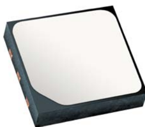
Figure 7. Si7021 with Factory-Installed Protective Cover
